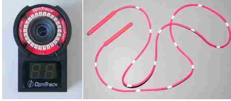
Figure 3.2: OptiTrack Flex camera(left), jump rope wrapped with reflective tape(right)
